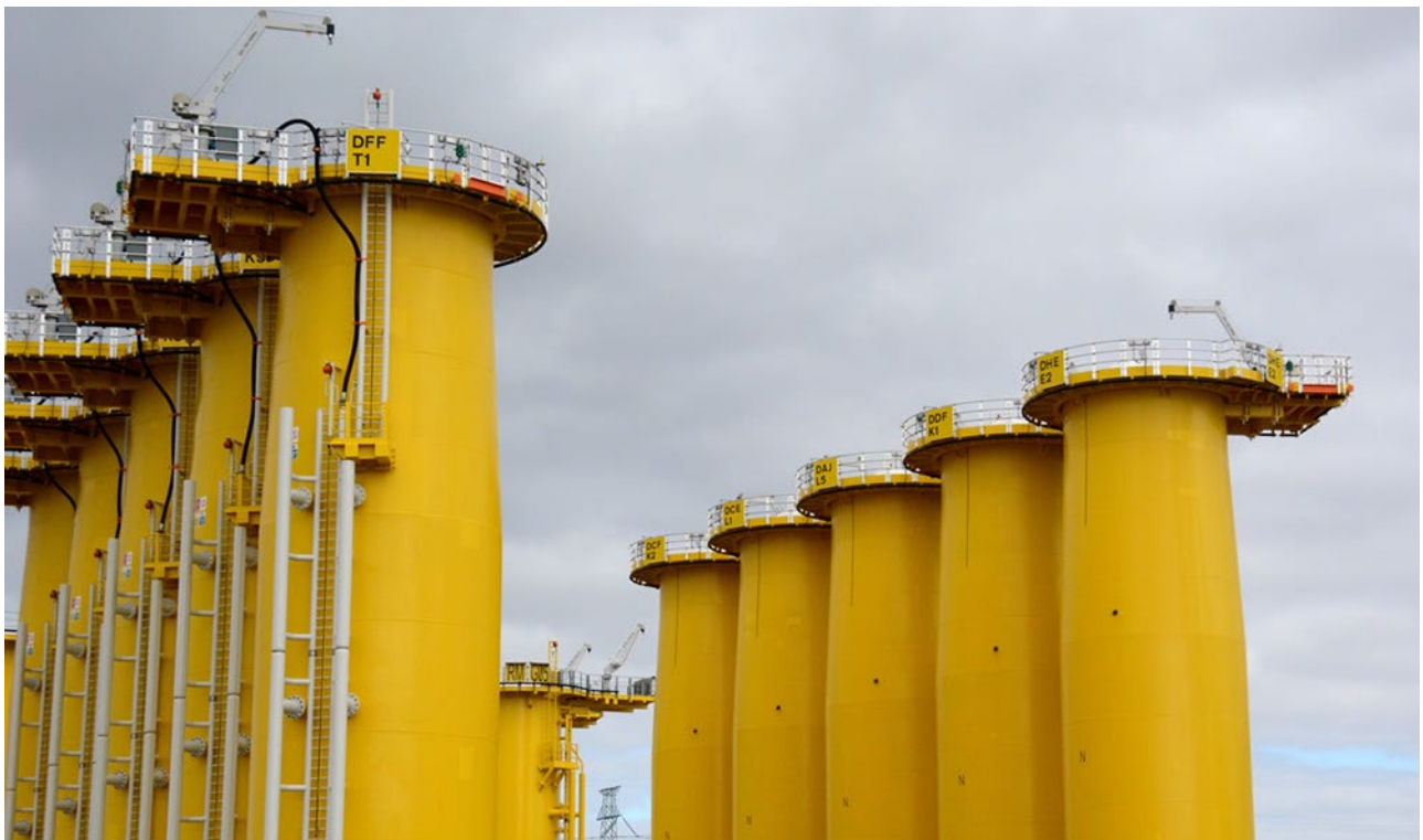
Plate 4-6: Monopile TPs ready for mobilisation to DOW (Source: Equinor)
