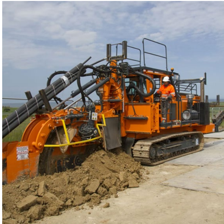
Plate 4-21: Example of cable trenching machine (Source: Equinor)
