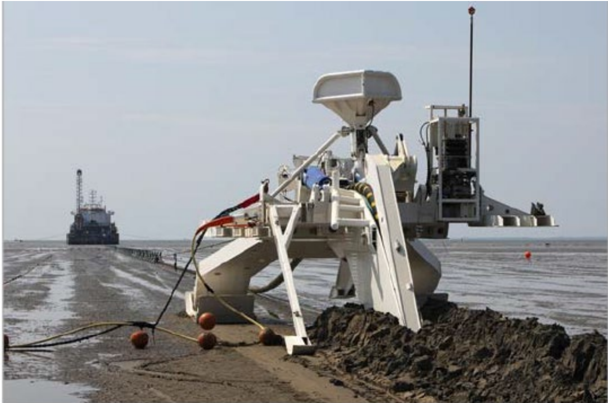
Plate 4-10: Example of a non-displacement plough (Source: Equinor)
